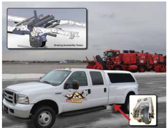
This vehicle, designed and built by the University of Waterloo and Team Eagle Ltd. can sense and monitor the affect of various contaminants on a facsimile aircraft braking system.
