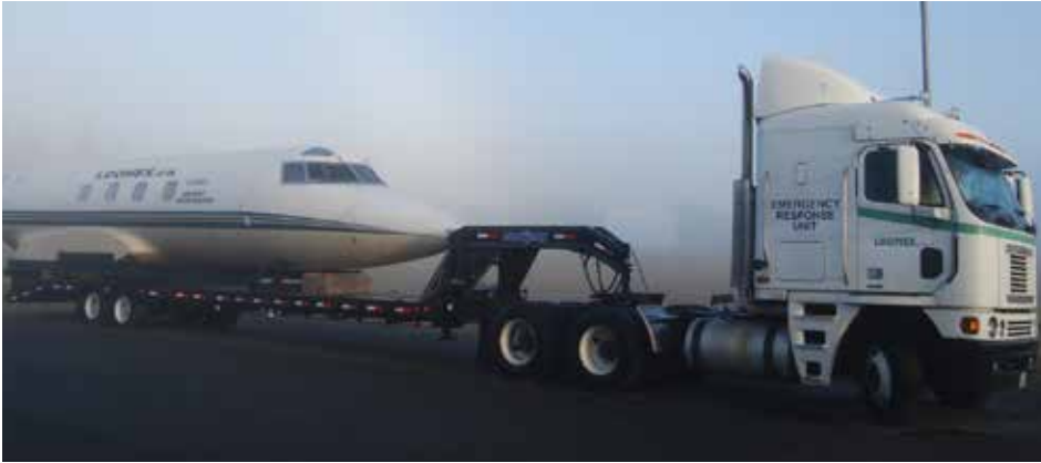
The team at The Loomex Group has created the country's only portable business jet crash site simulator using a Lockheed JetStar fuselage.
