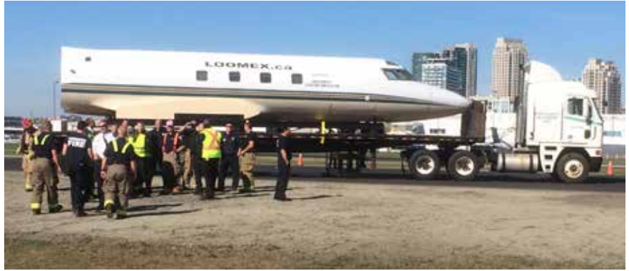
The Portable Simulator’s interior is finished as a private jet, and the bottom of the jet houses a cradle so it can be moved with a forklift.
