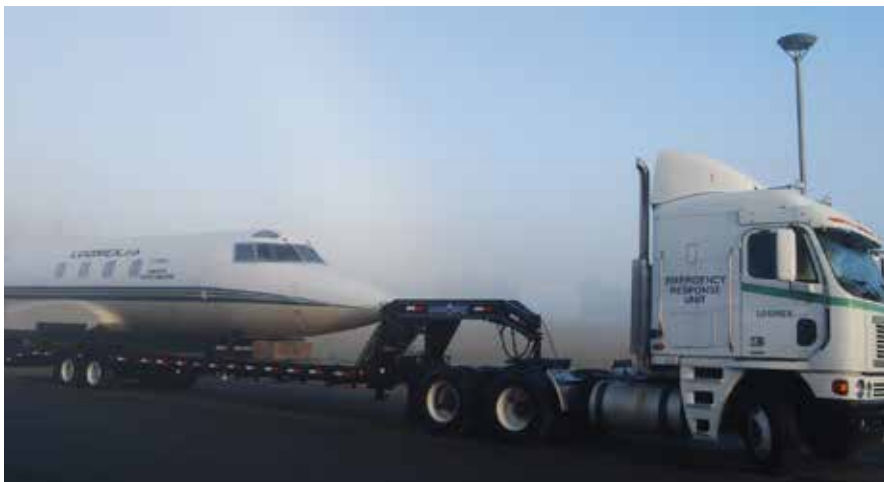
The team at the Loomex Group have created the country’s only portable business jet crash site simulator using a Lockheed JetStar fuselage.
